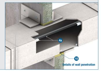
Self-supporting ducts provide an economical and fire safe method of constructing natural and mechanical smoke extract and ventilation ductwork without a steel lining. Lengths of the system can be prefabricated off-site or constructed on site using the applicable board type. This ensures that time spent on site is kept to a minimum, with little or no disruption to other trades.
